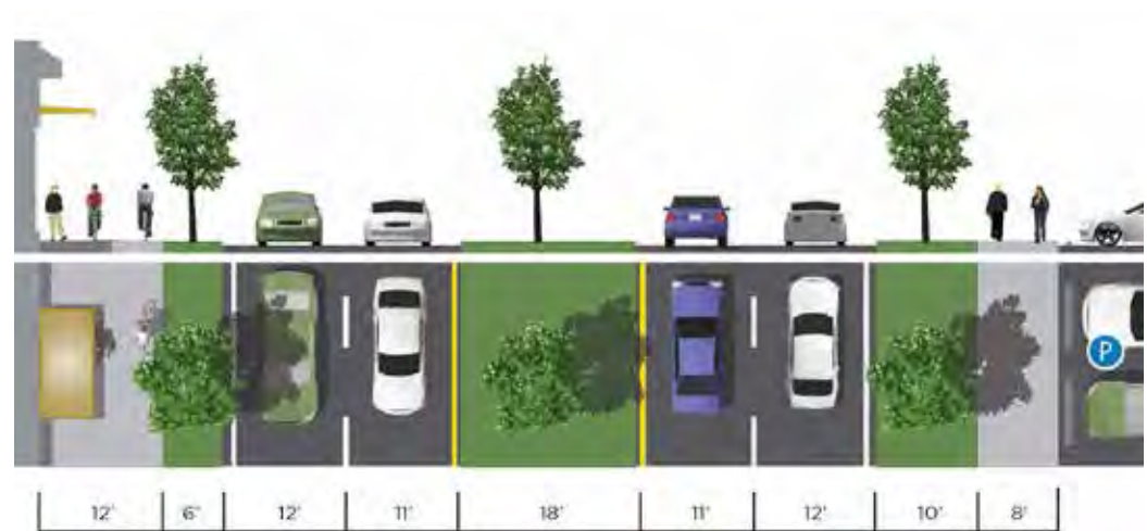
4-Lane Divided Boulevard Typical Section (Source: 2020 North Main Corridor Strategy Report)
