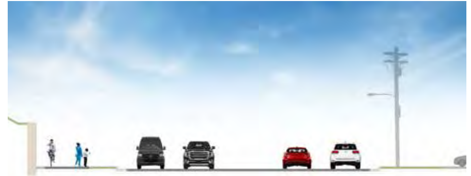
10' Sidepath + Retaining Wall
