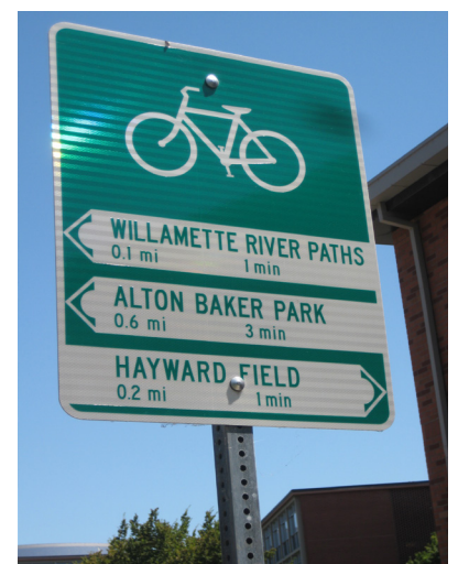
Bicycle wayfinding example that shows distance and time.
